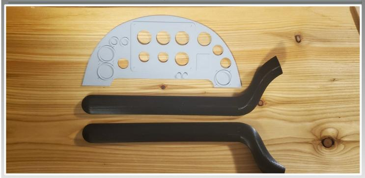
3D PRINT BY CARL LAYDEN: Panel and exhaust for Keith's Miles M20. Turned out well, Some time in CAD and about 15 hours on the printer. Used sketches from Keith as starting point. Exhaust is 9" long.
