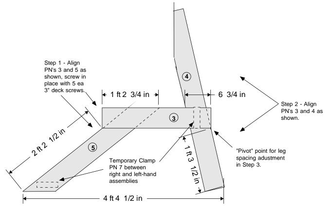
Step 3 - Adjust leg spacing to dimension shown by "pivoting" PN 4, and screw in place with 5 ea 3" deck screws.
